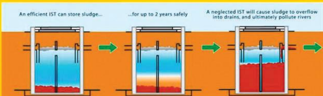
An Individual Septic Tank (or IST) which separates and stores the solid waste safely. The water then flows out into the drains.
