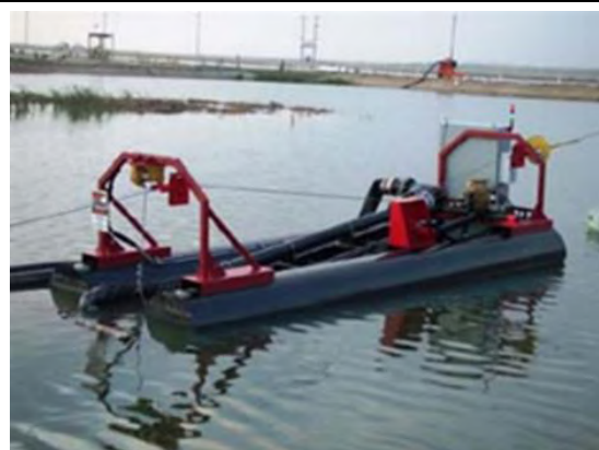
Figure A6.5: Dredging system for WSPs
