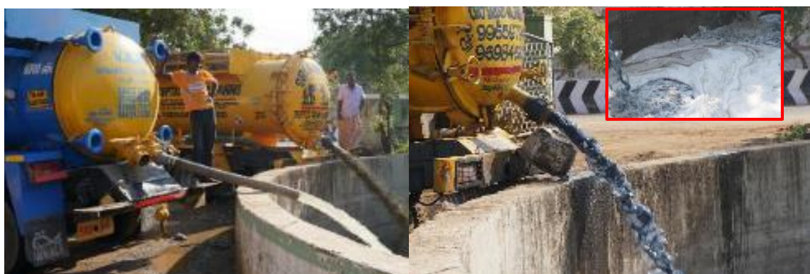
Figure 3.2: FS Disposal with no PPE and Non-Domestic Source of Sewage being Discharged
