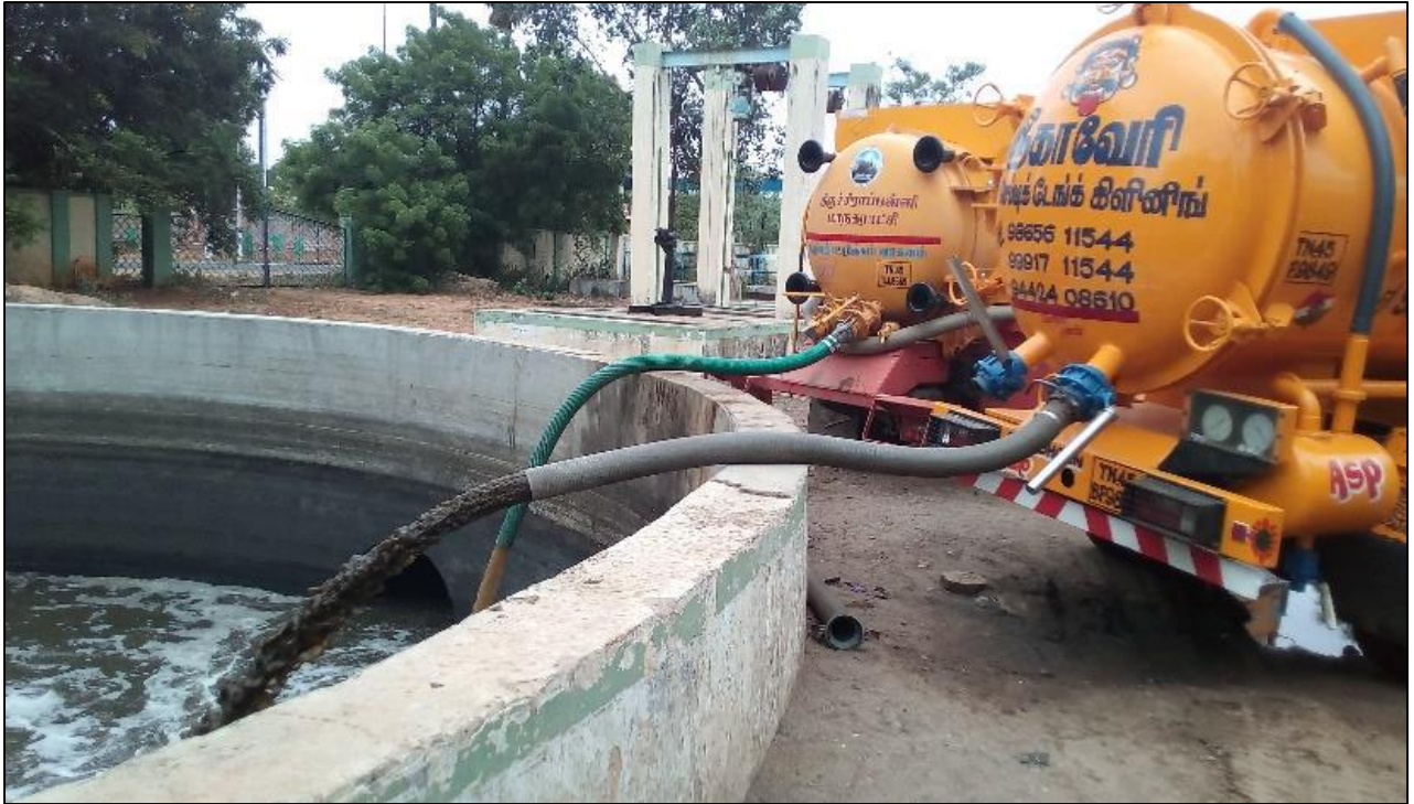
Figure A2.1: Photos of emptying FS/septage into collection well
