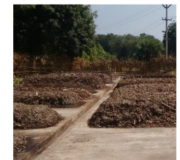
10. Co-composting of dried sludge with organic municipal solid waste
