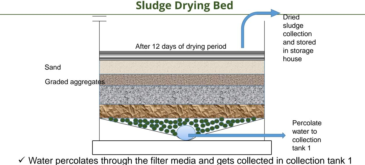
After 12 days of drying the sludge is collected and stored in sludge drying bed for co-composting
