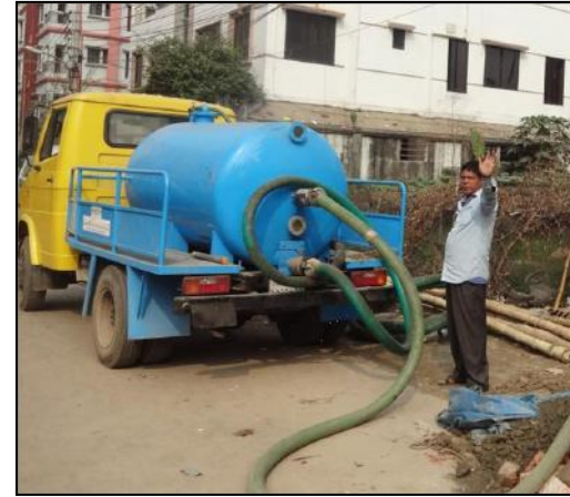
Emptying by vacuum pump (< 100 m sucking pipe) and truck
